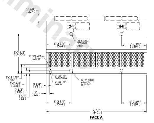
DRAWN BY: JLG SHIPPING NO. OF SHIPPING SECTIONS OPERATING HEAVIEST SECTION 9400 lbs+ [4265] kg+ 16340 lbs+ [7415] kg+ 6210 lbs+ [2820] kg+ WEIGHT WEIGHT WEIGHT
