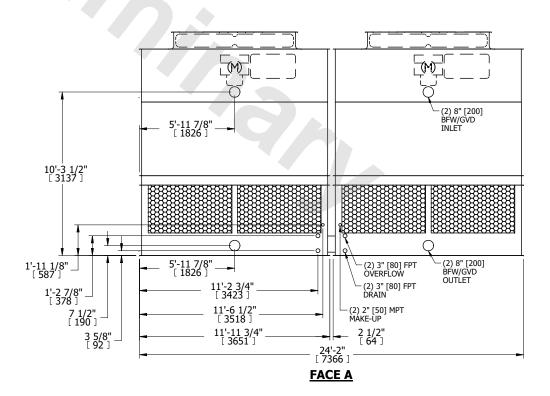
SHIPPING WEIGHT 12420 lbs+ [5635] kg+ OPERATING WEIGHT 20140 lbs+ [9140] kg+ HEAVIEST SECTION WEIGHT 4350 lbs+ [1975] kg+ NO. OF SHIPPING SECTIONS 4 DRAWN BY: JLG
