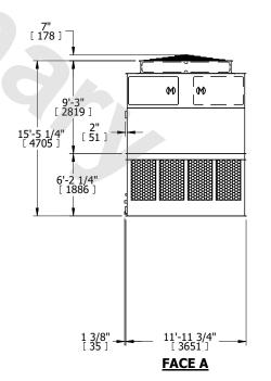
SHIPPING WEIGHT 14400 lbs+ [6535] kg+ OPERATING WEIGHT 24320 lbs+ [11035] kg+ HEAVIEST SECTION WEIGHT 4750 lbs+ [2155] kg+ NO. OF SHIPPING SECTIONS 4 DRAWN BY: KDS
