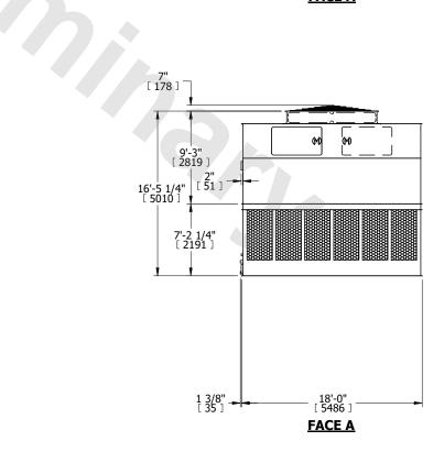
SHIPPING WEIGHT 20820 lbs+ [9445] kg+ OPERATING WEIGHT 36020 lbs+ [16340] kg+ HEAVIEST SECTION WEIGHT 6500 lbs+ [2950] kg+ NO. OF SHIPPING SECTIONS 4 DRAWN BY: JLG
