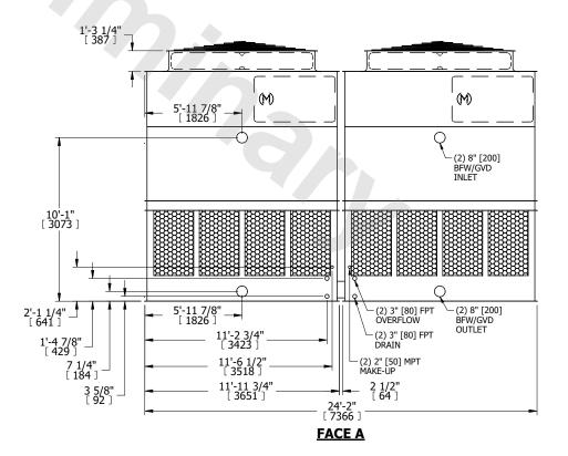
DRAWN BY: KDS NO. OF SHIPPING SECTIONS **SHIPPING** OPERATING HEAVIEST SECTION 14240 lbs+ [6460] kg+ 4680 lbs+ [2125] kg+ 24160 lbs+ [10960] kg+ WEIGHT WEIGHT WEIGHT
