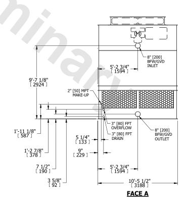
SHIPPING WEIGHT 5370 lbs+ [2440] kg+ OPERATING WEIGHT 8670 lbs+ [3935] kg+ HEAVIEST SECTION WEIGHT 3770 lbs+ [1715] kg+ NO. OF SHIPPING SECTIONS 2 DRAWN BY: JLG
