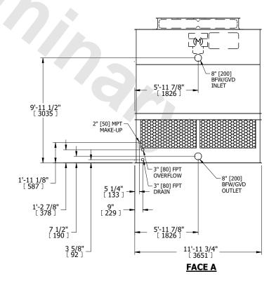
SHIPPING WEIGHT 6130 lbs+ [2785] kg+ OPERATING WEIGHT 9990 lbs+ [4535] kg+ HEAVIEST SECTION WEIGHT 4370 lbs+ [1985] kg+ NO. OF SHIPPING SECTIONS 2 DRAWN BY: JLG
