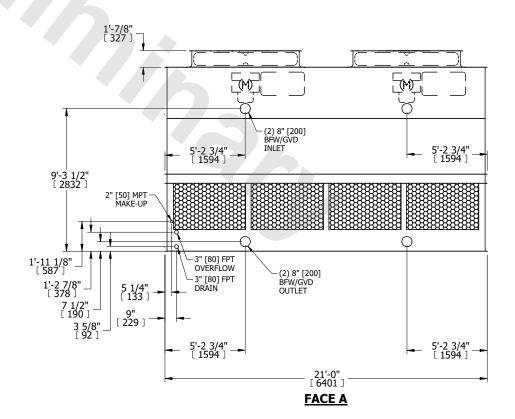
SHIPPING WEIGHT 10070 lbs+ [4570] kg+ OPERATING WEIGHT 17010 lbs+ [7720] kg+ HEAVIEST SECTION WEIGHT 6880 lbs+ [3125] kg+ NO. OF SHIPPING SECTIONS 2 DRAWN BY: JLG
