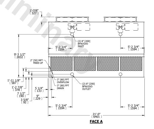
DRAWN BY: JLG SHIPPING NO. OF SHIPPING SECTIONS OPERATING HEAVIEST SECTION 10310 lbs+ [4680] kg+ 17250 lbs+ [7825] kg+ 7120 lbs+ [3230] kg+ WEIGHT WEIGHT WEIGHT
