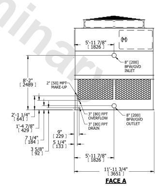
DRAWN BY: KDS NO. OF SHIPPING SECTIONS **SHIPPING** OPERATING HEAVIEST SECTION 7400 lbs+ [3360] kg+ 5000 lbs+ [2270] kg+ 13610 lbs+ [6175] kg+ WEIGHT WEIGHT WEIGHT
