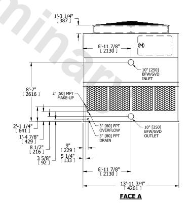
DRAWN BY: KDS NO. OF SHIPPING SECTIONS **SHIPPING** OPERATING HEAVIEST SECTION 8490 lbs+ [3855] kg+ 5620 lbs+ [2550] kg+ 15820 lbs+ [7180] kg+ WEIGHT WEIGHT WEIGHT
