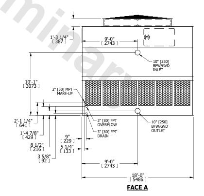
DRAWN BY: KDS NO. OF SHIPPING SECTIONS **SHIPPING** OPERATING HEAVIEST SECTION 11490 lbs+ [5215] kg+ 20760 lbs+ [9420] kg+ 7590 lbs+ [3445] kg+ WEIGHT WEIGHT WEIGHT
