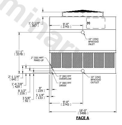
DRAWN BY: KDS SHIPPING NO. OF SHIPPING SECTIONS OPERATING HEAVIEST SECTION 12340 lbs+ [5600] kg+ 21610 lbs+ [9805] kg+ 8440 lbs+ [3830] kg+ WEIGHT WEIGHT WEIGHT
