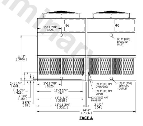
SHIPPING WEIGHT 17340 lbs+ [7870] kg+ OPERATING WEIGHT 29760 lbs+ [13500] kg+ HEAVIEST SECTION WEIGHT 6130 lbs+ [2785] kg+ NO. OF SHIPPING SECTIONS 4 DRAWN BY: KDS
