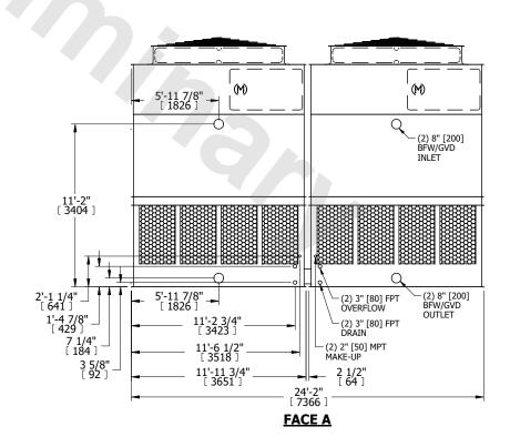
SHIPPING WEIGHT 18040 lbs+ [8185] kg+ OPERATING WEIGHT 30460 lbs+ [13820] kg+ HEAVIEST SECTION WEIGHT 6480 lbs+ [2940] kg+ NO. OF SHIPPING SECTIONS 4 DRAWN BY: KDS
