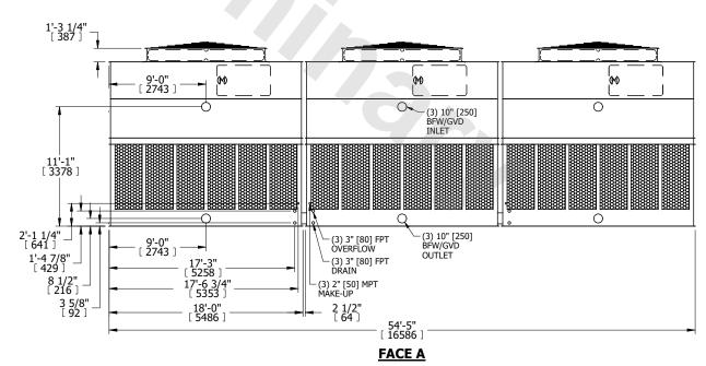
SHIPPING WEIGHT 33300 lbs+ [15105] kg+ OPERATING WEIGHT 61110 lbs+ [27720] kg+ HEAVIEST SECTION WEIGHT 6920 lbs+ [3140] kg+ NO. OF SHIPPING SECTIONS 6 DRAWN BY: KDS
