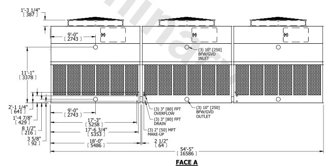
DRAWN BY: KDS NO. OF SHIPPING SECTIONS **SHIPPING** OPERATING HEAVIEST SECTION 34080 lbs+ [15460] kg+ 61890 lbs+ [28075] kg+ 7180 lbs+ [3260] kg+ WEIGHT WEIGHT WEIGHT
