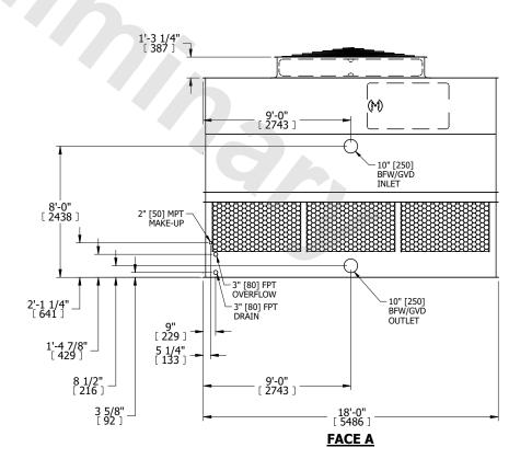
SHIPPING WEIGHT 9460 lbs+ [4295] kg+ OPERATING WEIGHT 17060 lbs+ [7740] kg+ HEAVIEST SECTION WEIGHT 5910 lbs+ [2685] kg+ NO. OF SHIPPING SECTIONS 2 DRAWN BY: KDS
