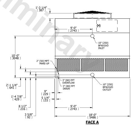
SHIPPING WEIGHT 10780 lbs+ [4890] kg+ OPERATING WEIGHT 18380 lbs+ [8340] kg+ HEAVIEST SECTION WEIGHT 7230 lbs+ [3280] kg+ NO. OF SHIPPING SECTIONS 2 DRAWN BY: KDS
