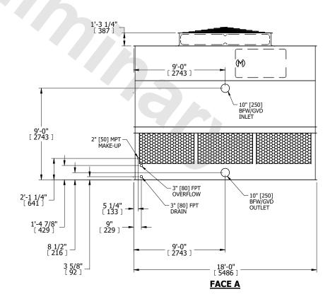
DRAWN BY: JLG NO. OF SHIPPING SECTIONS **SHIPPING** OPERATING HEAVIEST SECTION 10400 lbs+ [4720] kg+ 18000 lbs+ [8165] kg+ 6850 lbs+ [3110] kg+ WEIGHT WEIGHT WEIGHT
