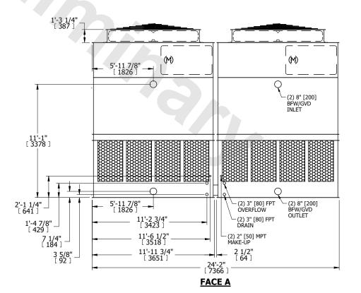
SHIPPING WEIGHT 16120 lbs+ [7315] kg+ OPERATING WEIGHT 26040 lbs+ [11815] kg+ HEAVIEST SECTION WEIGHT 5620 lbs+ [2550] kg+ NO. OF SHIPPING SECTIONS 4 DRAWN BY: JLG
