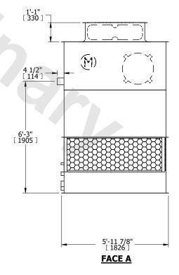
DRAWN BY: KWC NO. OF SHIPPING SECTIONS **SHIPPING** OPERATING HEAVIEST SECTION 1390 lbs+ [635] kg+ 2410 lbs+ [1095] kg+ 950 lbs+ [435] kg+ WEIGHT WEIGHT WEIGHT
