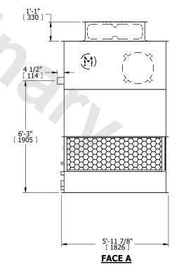
DRAWN BY: KWC NO. OF SHIPPING SECTIONS **SHIPPING** OPERATING HEAVIEST SECTION 1410 lbs+ [640] kg+ 2430 lbs+ [1105] kg+ 970 lbs+ [440] kg+ WEIGHT WEIGHT WEIGHT
