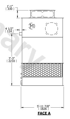
SHIPPING WEIGHT 1510 lbs+ [685] kg+ OPERATING WEIGHT 2530 lbs+ [1150] kg+ HEAVIEST SECTION WEIGHT 1070 lbs+ [490] kg+ NO. OF SHIPPING SECTIONS 2 DRAWN BY: KWC
