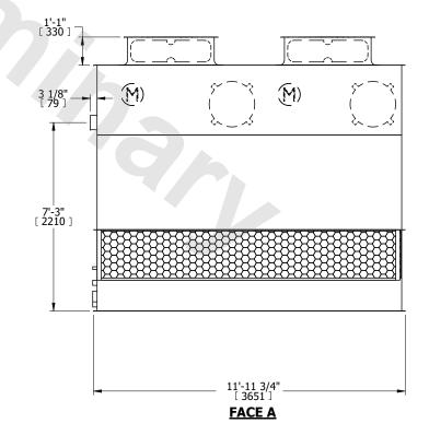
SHIPPING WEIGHT 2730 lbs+ [1240] kg+ OPERATING WEIGHT 4850 lbs+ [2200] kg+ HEAVIEST SECTION WEIGHT 1970 lbs+ [895] kg+ NO. OF SHIPPING SECTIONS 2 DRAWN BY: KWC
