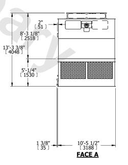
SHIPPING WEIGHT 10280 lbs+ [4665] kg+ OPERATING WEIGHT 16880 lbs+ [7660] kg+ HEAVIEST SECTION WEIGHT 3420 lbs+ [1555] kg+ NO. OF SHIPPING SECTIONS 4 DRAWN BY: KDS
