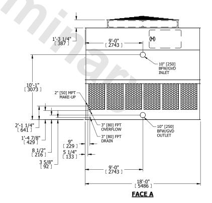
DRAWN BY: KDS NO. OF SHIPPING SECTIONS **SHIPPING** OPERATING HEAVIEST SECTION 11440 lbs+ [5190] kg+ 20710 lbs+ [9395] kg+ 7540 lbs+ [3425] kg+ WEIGHT WEIGHT WEIGHT
