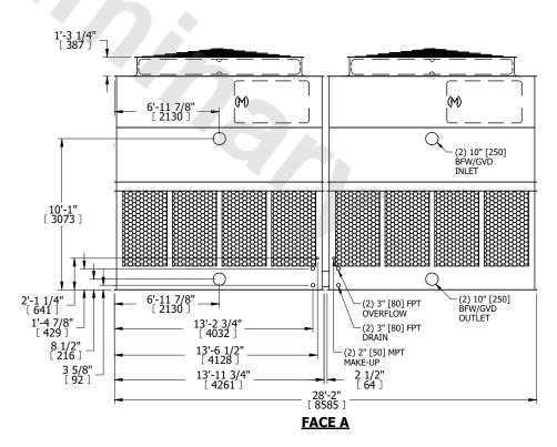
SHIPPING WEIGHT 17080 lbs+ [7750] kg+ OPERATING WEIGHT 31740 lbs+ [14400] kg+ HEAVIEST SECTION WEIGHT 5490 lbs+ [2495] kg+ NO. OF SHIPPING SECTIONS 4 DRAWN BY: KDS
