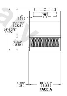
SHIPPING WEIGHT 10980 lbs+ [4985] kg+ OPERATING WEIGHT 17580 lbs+ [7975] kg+ HEAVIEST SECTION WEIGHT 3770 lbs+ [1715] kg+ NO. OF SHIPPING SECTIONS 4 DRAWN BY: KDS
