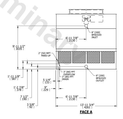
SHIPPING WEIGHT 6760 lbs+ [3070] kg+ OPERATING WEIGHT 11270 lbs+ [5115] kg+ HEAVIEST SECTION WEIGHT 4710 lbs+ [2140] kg+ NO. OF SHIPPING SECTIONS 2 DRAWN BY: JLG
