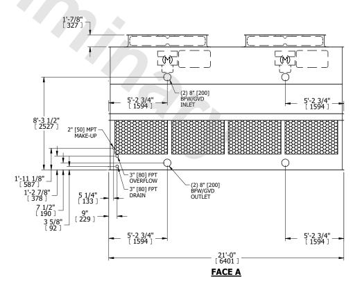
SHIPPING WEIGHT 9460 lbs+ [4295] kg+ OPERATING WEIGHT 16400 lbs+ [7440] kg+ HEAVIEST SECTION WEIGHT 6270 lbs+ [2845] kg+ NO. OF SHIPPING SECTIONS 2 DRAWN BY: JLG
