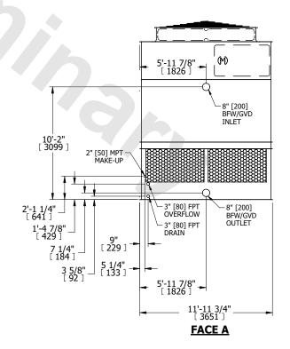
SHIPPING WEIGHT 8530 lbs+ [3870] kg+ OPERATING WEIGHT 14740 lbs+ [6690] kg+ HEAVIEST SECTION WEIGHT 6130 lbs+ [2785] kg+ NO. OF SHIPPING SECTIONS 2 DRAWN BY: KDS
