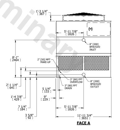
SHIPPING WEIGHT 6690 lbs+ [3035] kg+ OPERATING WEIGHT 11650 lbs+ [5285] kg+ HEAVIEST SECTION WEIGHT 4270 lbs+ [1940] kg+ NO. OF SHIPPING SECTIONS 2 DRAWN BY: JLG
