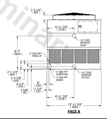
DRAWN BY: KDS NO. OF SHIPPING SECTIONS OPERATING HEAVIEST SECTION 8230 lbs+ [3735] kg+ 5360 lbs+ [2435] kg+ 15560 lbs+ [7060] kg+ WEIGHT WEIGHT
