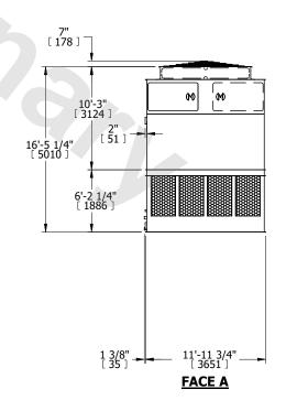
SHIPPING WEIGHT 15240 lbs+ [6915] kg+ OPERATING WEIGHT 25160 lbs+ [11415] kg+ HEAVIEST SECTION WEIGHT 5170 lbs+ [2350] kg+ NO. OF SHIPPING SECTIONS
