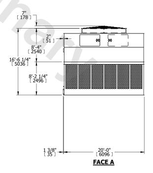
SHIPPING WEIGHT 23660 lbs+ [10735] kg+ OPERATING WEIGHT 44460 lbs+ [20170] kg+ HEAVIEST SECTION WEIGHT 7210 lbs+ [3275] kg+ NO. OF SHIPPING SECTIONS 4 DRAWN BY: BLL
