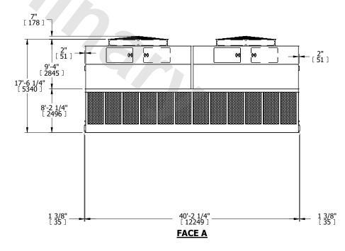
DRAWN BY: BLL NO. OF SHIPPING SECTIONS **SHIPPING** OPERATING HEAVIEST SECTION 51440 lbs+ [23335] kg+ 92640 lbs+ [42025] kg+ 9000 lbs+ [4085] kg+ WEIGHT WEIGHT WEIGHT
