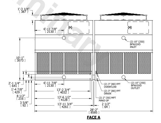
SHIPPING WEIGHT 16820 lbs+ [7630] kg+ OPERATING WEIGHT 31480 lbs+ [14280] kg+ HEAVIEST SECTION WEIGHT 5360 lbs+ [2435] kg+ NO. OF SHIPPING SECTIONS 4 DRAWN BY: KDS
