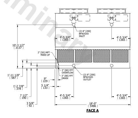
SHIPPING WEIGHT 9300 lbs+ [4220] kg+ OPERATING WEIGHT 15190 lbs+ [6895] kg+ HEAVIEST SECTION WEIGHT 6480 lbs+ [2940] kg+ NO. OF SHIPPING SECTIONS 2 DRAWN BY: JLG
