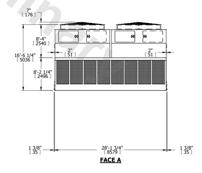
SHIPPING WEIGHT 34260 lbs+ [15545] kg+ OPERATING WEIGHT 63160 lbs+ [28650] kg+ HEAVIEST SECTION WEIGHT 6550 lbs+ [2975] kg+ NO. OF SHIPPING SECTIONS 6 DRAWN BY: JLG
