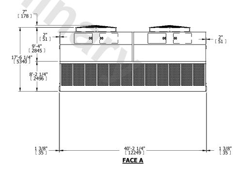
SHIPPING WEIGHT 50400 lbs+ [22865] kg+ OPERATING WEIGHT 91600 lbs+ [41550] kg+ HEAVIEST SECTION WEIGHT 9000 lbs+ [4085] kg+ NO. OF SHIPPING SECTIONS 6 DRAWN BY: BLL
