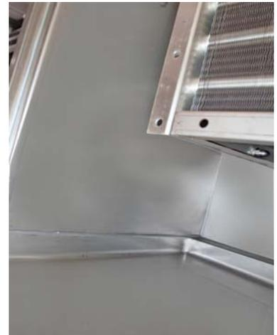
The coil(s) for ammonia use shall be constructed using 0.025" wall stainless tubes and 0.014 thick aluminum fins (maximum of 8 FPI). Coil shall meet strength requirements of ASME/ANSI B31.5. All coils shall be charged with nitrogen prior to shipment. Coil performance shall be rated in accordance with AHRI 420.
