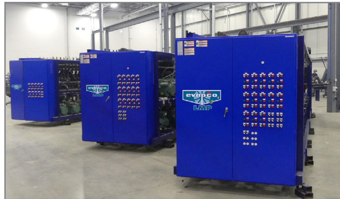
Purity Rack Highlighting Microprocessor Control Panels
