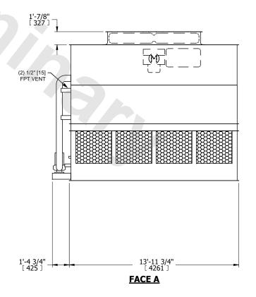
SHIPPING WEIGHT 16250 lbs+ [7375] kg+ OPERATING WEIGHT 23220 lbs+ [10535] kg+ HEAVIEST SECTION WEIGHT 14170 lbs+ [6430] kg+ NO. OF SHIPPING SECTIONS 2 DRAWN BY: JLG
