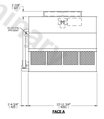
SHIPPING WEIGHT 16300 lbs+ [7395] kg+ OPERATING WEIGHT 23270 lbs+ [10560] kg+ HEAVIEST SECTION WEIGHT 14220 lbs+ [6455] kg+ NO. OF SHIPPING SECTIONS 2 DRAWN BY: JLG
