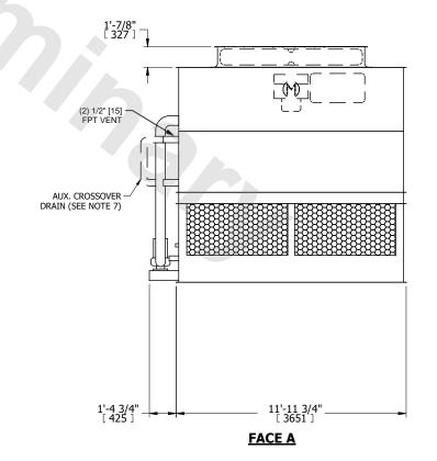
DRAWN BY: JLG NO. OF SHIPPING SECTIONS **SHIPPING** OPERATING HEAVIEST SECTION 14090 lbs+ [6395] kg+ 20080 lbs+ [9110] kg+ 12220 lbs+ [5545] kg+ WEIGHT WEIGHT WEIGHT
