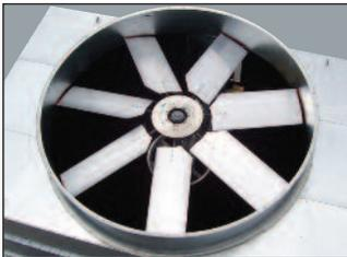
The Low Sound Fan is capable of reducing the unit sound pressure levels by **4 dB(A) to 7dB(A)**, depending on specific unit selection and measurement location with a minimal impact to thermal performance. The fans are high efficiency axial propeller type.
