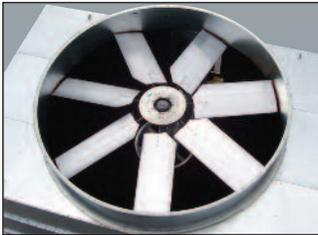
The Low Sound Fan offered by EVAPCO uses a wide chord blade design for sound sensitive applications where low sound levels are desired. Low Sound Fan construction uses aluminum blades and a steel fan hub. The Low Sound Fan is capable of reducing the unit sound pressure levels by **4 dB(A) to 7dB(A)**, depending on specific unit selection and measurement location
