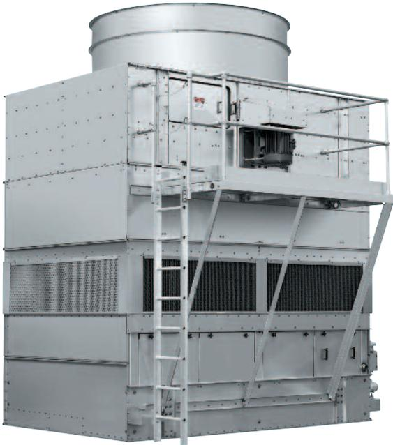
External platforms provide a sturdy base for access to the drive components, water distribution and drift eliminators. Constructed from heavy gauge galvanized steel, the platform mounts easily to the unit and requires no external support. The platform option includes a vertical aluminum ladder and meets all applicable OSHA requirements. A safety cage for the ladder is also available if required for the installation.
