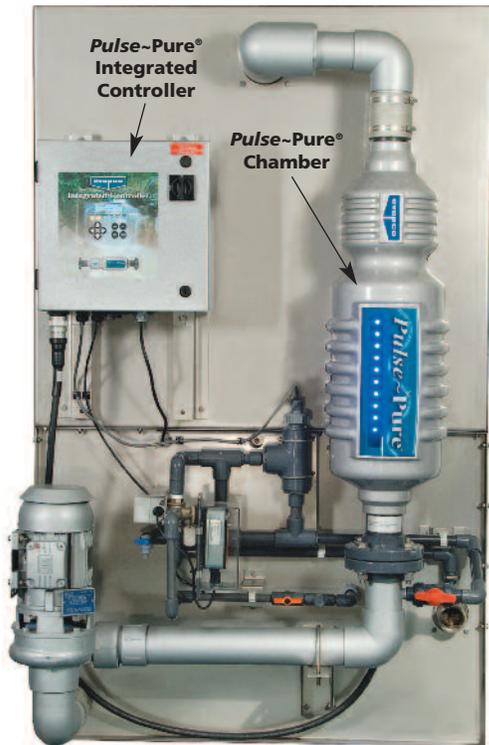
EVAPCO's **Pulse~Pure®** water treatment system utilizes pulsed electric field technology to provide an environmentally responsible alternative for the treatment of water in evaporative cooled equipment. The **Pulse~Pure®** system delivers short, high-frequency bursts of low energy electromagnetic fields to the recirculating water in the ESWA.
