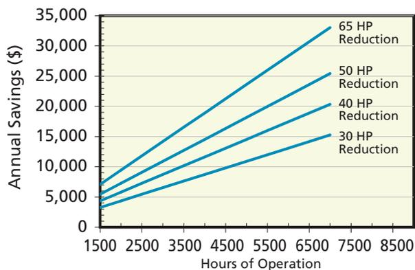
Annual savings based on fan motor efficiency = 0.924 and energy cost of \$0.09/kWh
