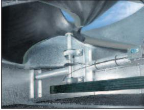
The Super Low Sound Fan offered by EVAPCO uses an extremely wide chord blade design for very sound sensitive applications where the lowest sound levels are required. The fan is one-piece molded heavy duty FRP construction utilizing a forward swept blade design.
