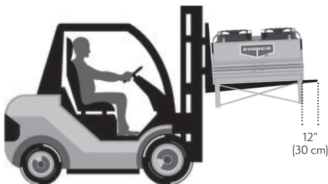
Figure 4 – Flat Coil Unit Forklift Lifting Requirements
