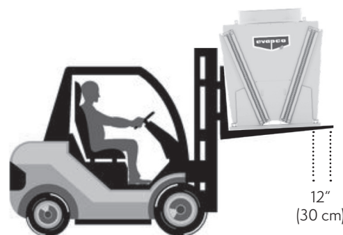
Figure 12 – V-Coil Unit Forklift Lifting Requirements
