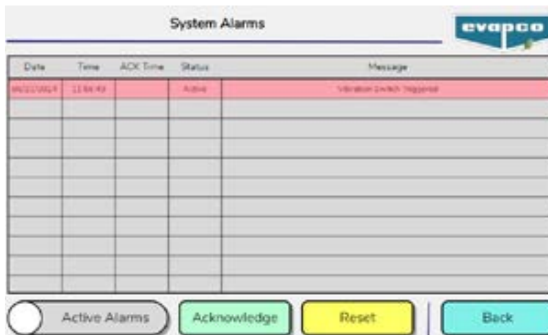
Figure 17 - Alarms Screen with Active Alarm
