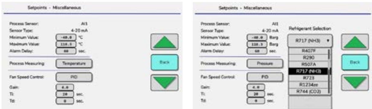
Figure 29 - Process Measuring Set to Temperature for Fluid Coolers and Pressure for Condensers
