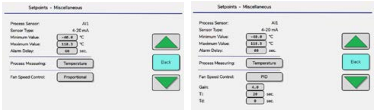
Figure 31 - Proportional or PID Fan Speed Control Setting
