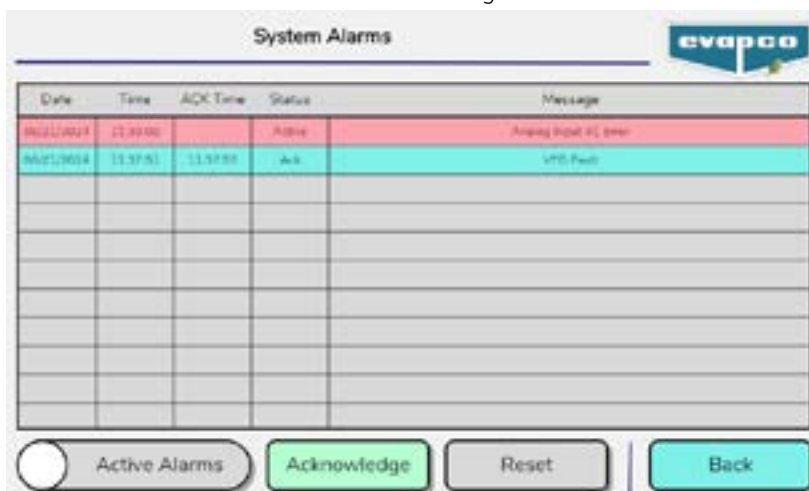
Figure 15 - Active Alarm Screen
