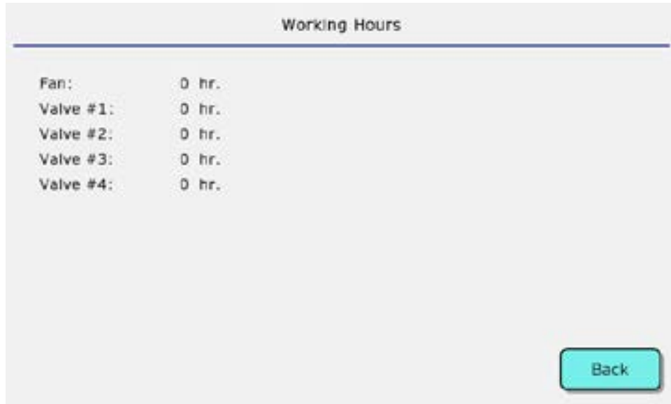
Figure 43 - Fan and Solenoid Valves Working Hours
